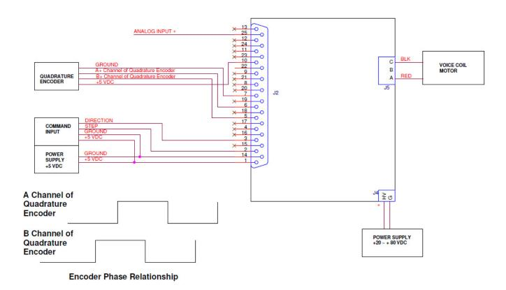
DC MOTOR CONTROL with STEP and DIRECTION COMMAND INPUT or ANALOG INPUT
